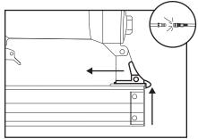
Figure 3. Pressing the magazine latch.
